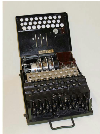
Figure 1: Three rotor Enigma I Machine on display at the Bletchley Park museum
